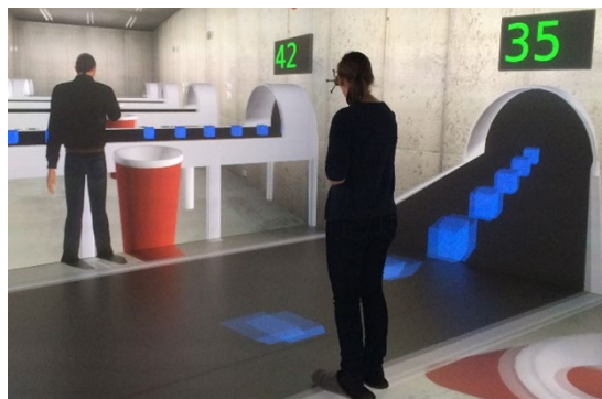
Figure 1: A subject, in the foreground, working on the conveyer belt task in the aixCAVE of RWTH Aachen University in the presence of a virtual co-worker. The virtual counters on the wall display running tallies of the avatar’s and the test subject’s accumulated performance points. In this picture, projected objects appear double and overlaying because of the stereoscopic projection. For the participant in the foreground, who is wearing 3D glasses, the projection is distinct, and the cube in front of her appears to be at the level of her waist.
